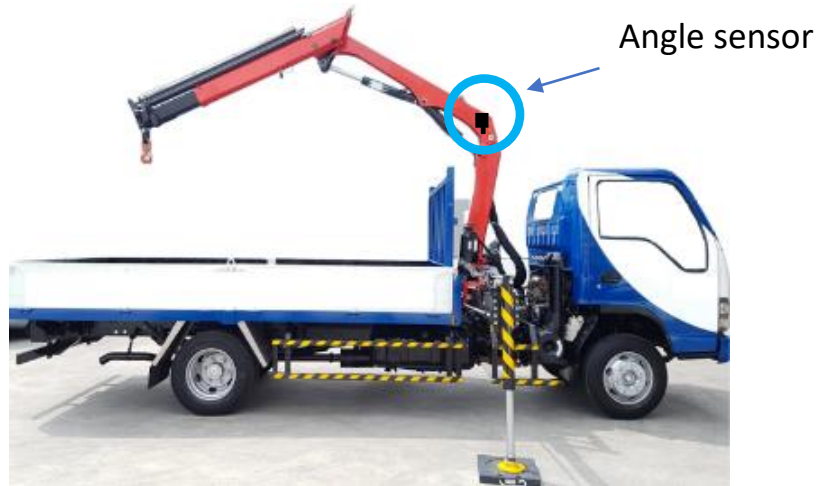
Inner boom more than 90° (above maximum stowed height), buzzer will activate
