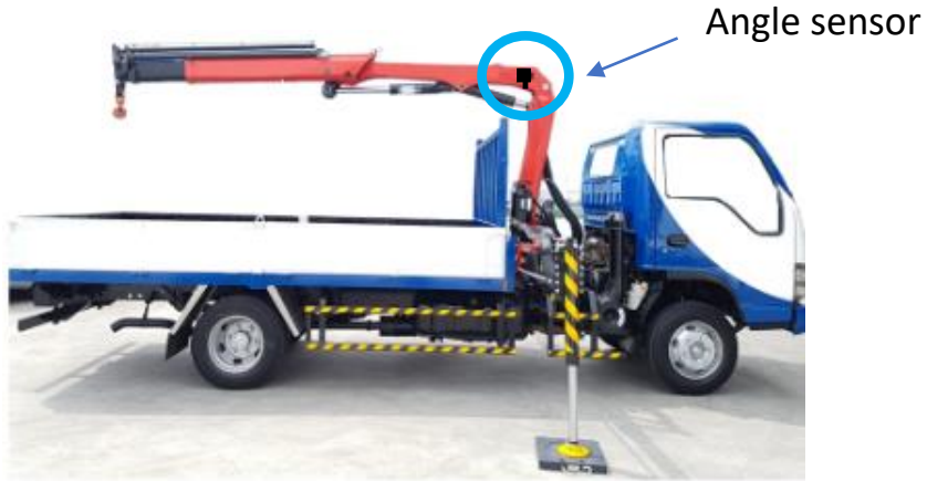
Inner boom not greater than 90°, buzzer will not activate
