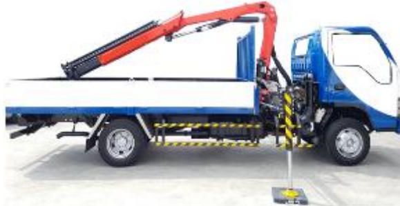
Positions of Crane Boom (AWS Activated)
